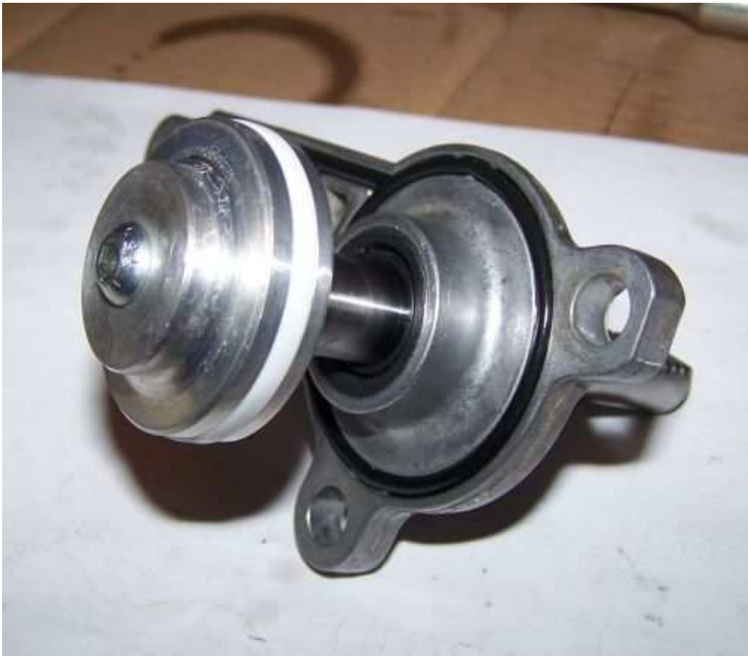
The heart of the control mechanism of the HCU is the “spool valve”, this looks like a pipe which is full of holes.
