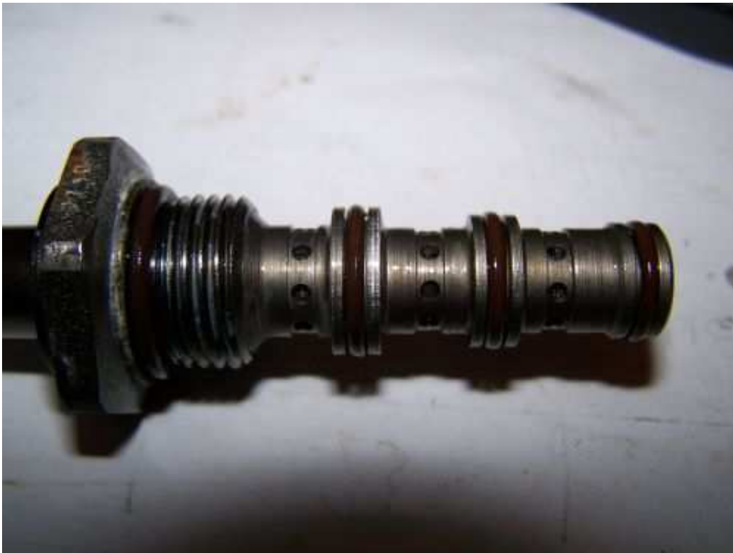
The heart of the control mechanism of the HCU is the “spool valve”, this looks like a pipe which is full of holes.
